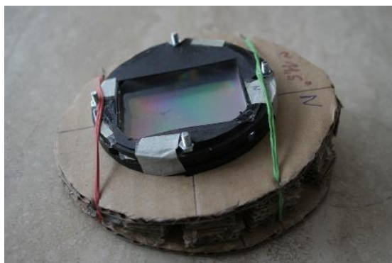
Fig. 17: Objective grating wedge for a tilt angle of 12^\circ .
